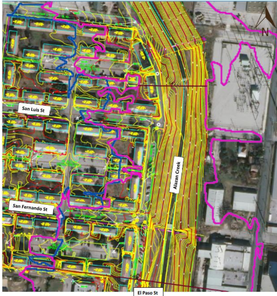
Figure 2 – LOMR Topographic Workmap / Existing and Modified Floodplain
